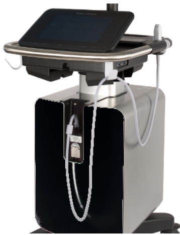
Transducer bay with transducer connected
