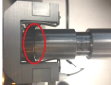
Transducer ferrule that is pushed all the way in to the port.
