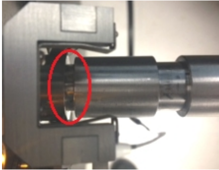
Transducer ferrule that is not pushed all the way in to the port.
